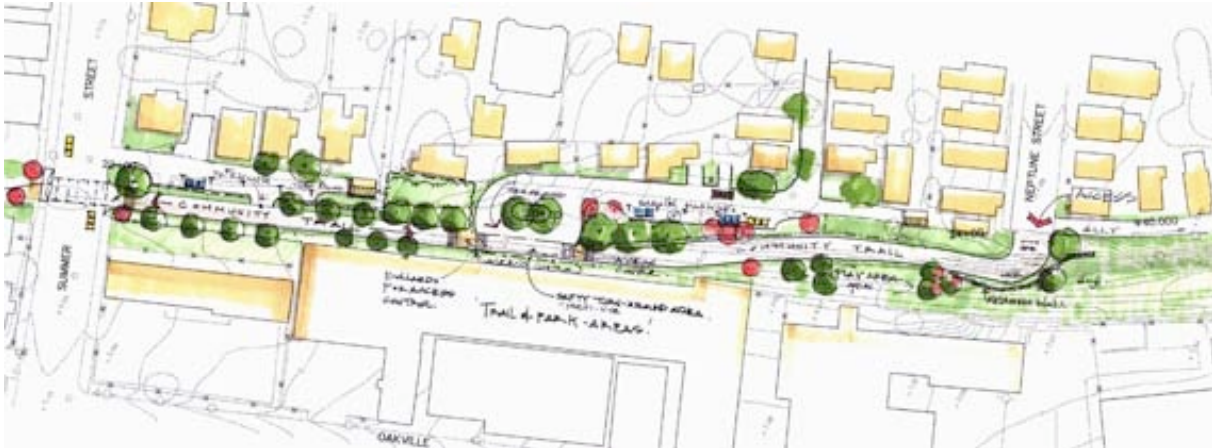
Possible design solution for the proposed Lynn section of the Northern Strand Community trail
